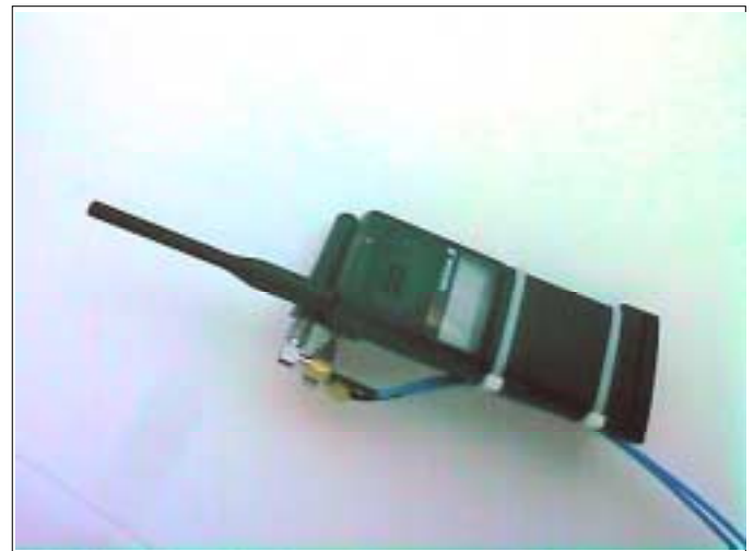
Figure 3 - Commercially available handset, modified with second antenna
