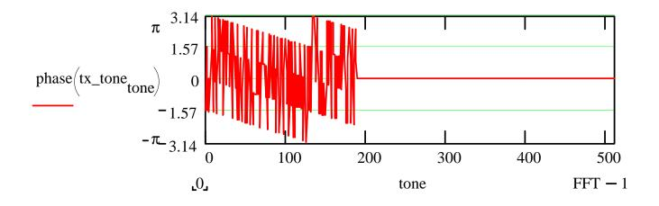
At the receiver, each transmit tone phase is shifted by an amount proportional to the tone frequency and the timing offset (by the Fourier Transform shifting property)
