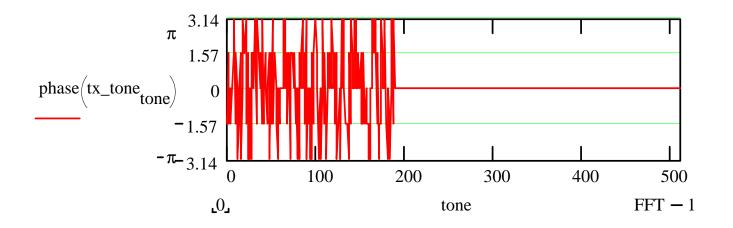
Transmitter generates a set of QPSK modulated tones - the phase of each tone is a multiple of  $\pi/2$
