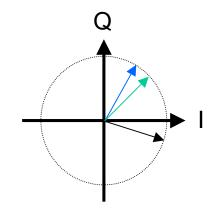
Each tone phase is differentially detected (in frequency) with respect to its neighbor
