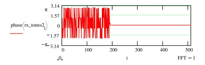
At the receiver, each transmit tone phase is shifted proportionally to frequency offset, plus some frequency dependent phase modulation, due to "beating" between tones
